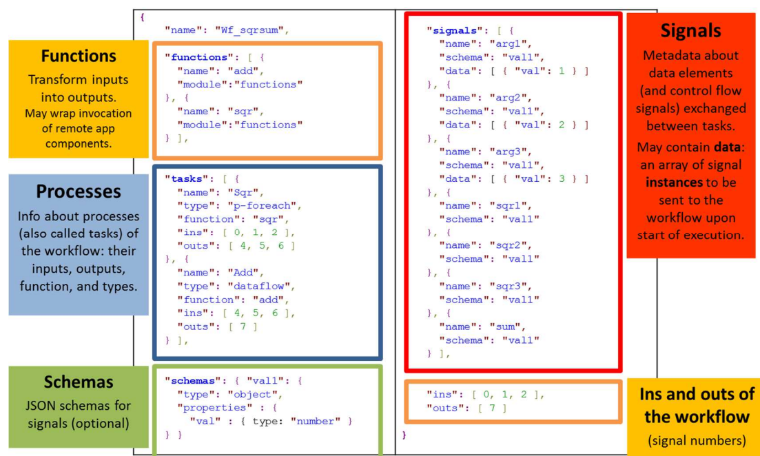
Figure 2: Specification of the sum of squares workflow in the HyperFlow format.
